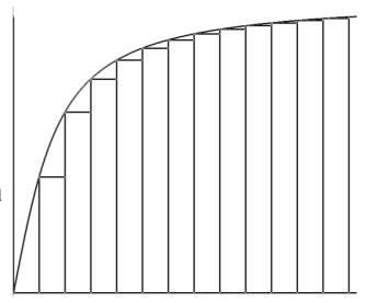
starting temperature which each timestep would just compare their temperature to the temperature of the points around it and then transfer some of it's heat energy to those surrounding nodes proportional to the temperature difference.
